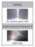
Result: EMP09 series of tangential milling cutter has higher precision and better surface quality, no obvious gear mark, and runout value, which is better than the similar product of company A. 20 15 10 5 0 AN11 AN15
