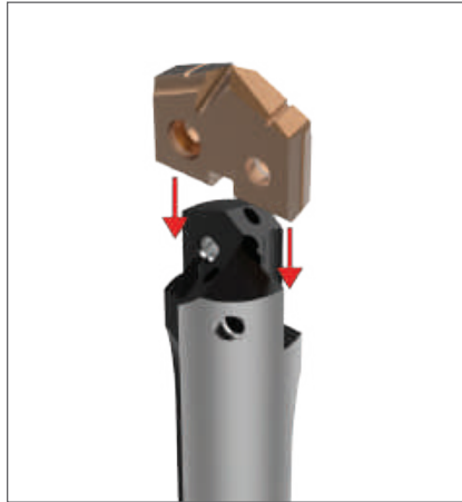
Step 1: Align the flats on the T-A Pro insert with the flats on the ears of the holder.
